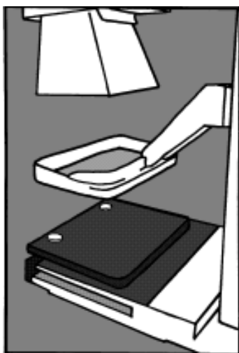
Fig. 2.3 Alignment of X-ray field/image receptor measurement
