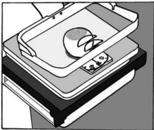
Fig. 2.4 Compression force measurement
